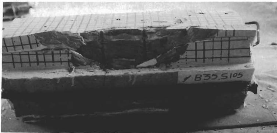
Figure 9.5 a) Block after blasting, with joints dipping away from the face and joints are parallel to face and b) Blocks after blasting with joints dipping into the face and joints are parallel to face.
