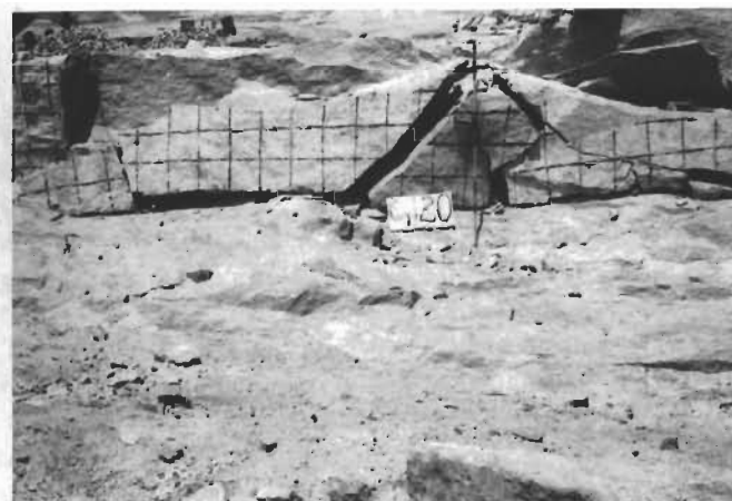
Figure 8.11 Development of cracks in large fragment in quarry test.
