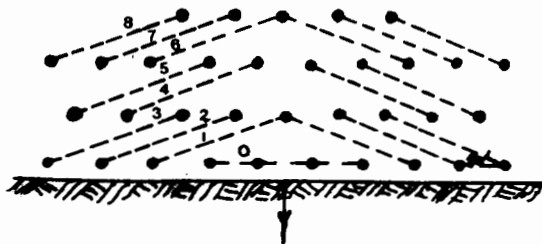
Figure 11.11 Multihole/multirow blasting with various delay patterns.
