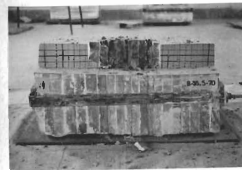
Figure 9.6 a) Perpendicular bedding planes steeply dipping up direction in a limestone quarry, b) Top view of reassembled fragments for perpendicular vertical joints, c) Front view of reassembled fragments for perpendicular steeply dipping jointed blocks.
