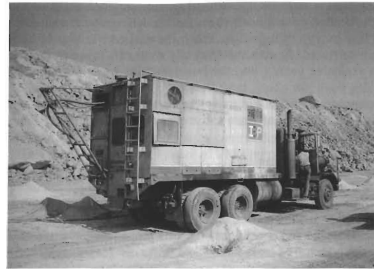
Figure 4.6 Site Mixed slurry/emulsion explosive loading truck (courtesy IBP Co.).
