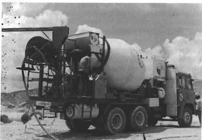
Figure 4.7 Plant mixed slurry explosive loading truck (courtesy Indo-Gulf).
