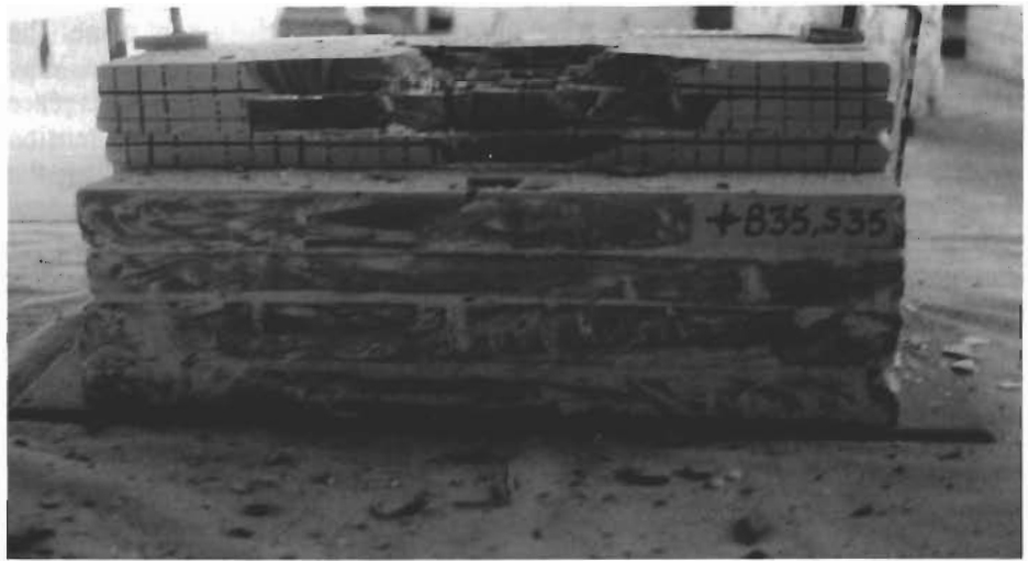
Figure 8.17 Blasted block with horizontal joints. a) Top view of reassembled fragments for horizontal joints (showing fracture pattern and b) Front view of reassembled fragments for horizontal joints.
