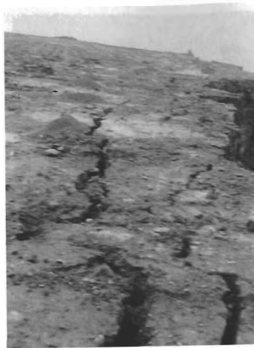
Figure 20.1 Damage to remaining rock after a blast in an open pit mine.
