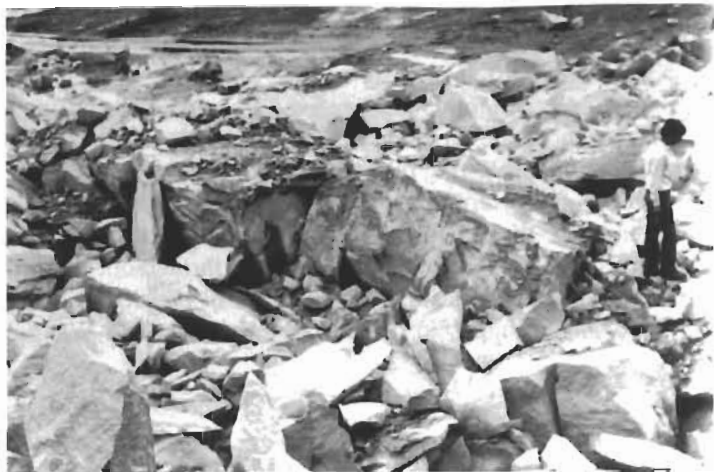
Figure 16.3 Fragmentation during armour stone production.
